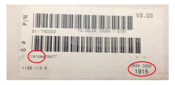
The image on the previous page shows the date code of the thermostat. The date code pictured was built on the 19<sup>th</sup> week of 2015. If this thermostat happened to be a new thermostat that has not been installed or will not be installed by June 15<sup>th</sup> 2016 and connected to a WIFI internet connection, then it will never be able to connect to WIFI. However it will still function as a thermostat, just not WIFI capable.
